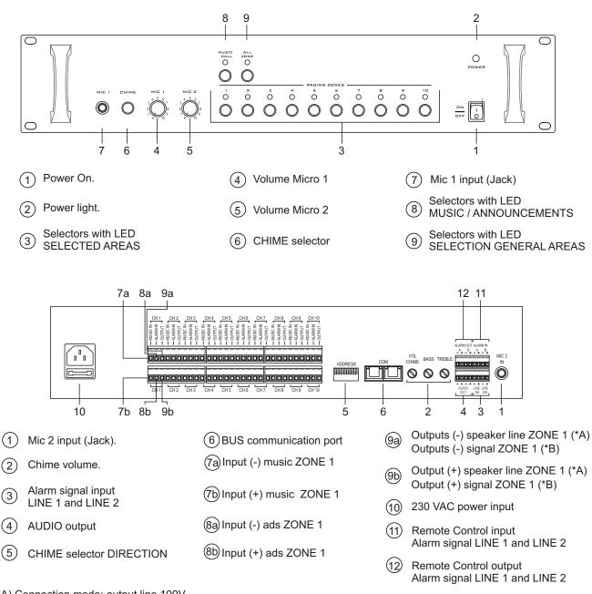
(\*A) Connection mode: output line 100V
