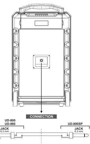
2 cables with a minimum cross-section of 1.5 mm<sup>2</sup> for distances shorter than 20 metres
