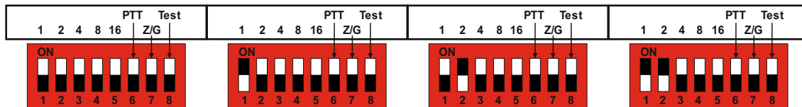
Values assigned to each DIP switch
