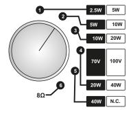
**Warning:** If the loudspeaker is connected to L100V, do not set the switch to position 5 and 6 under any circumstances. It will cause damage to the loudspeaker and the power amplifier to which it is connected.
