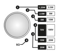
Warning: If the loudspeaker is connected to L100V, do not set the switch to position 5 and 6 under any circumstances. It will cause damage to the loudspeaker and the power amplifier to which it is connected.
