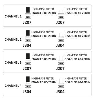
The factory setting is with the filter on 80Hz-20KHz.
