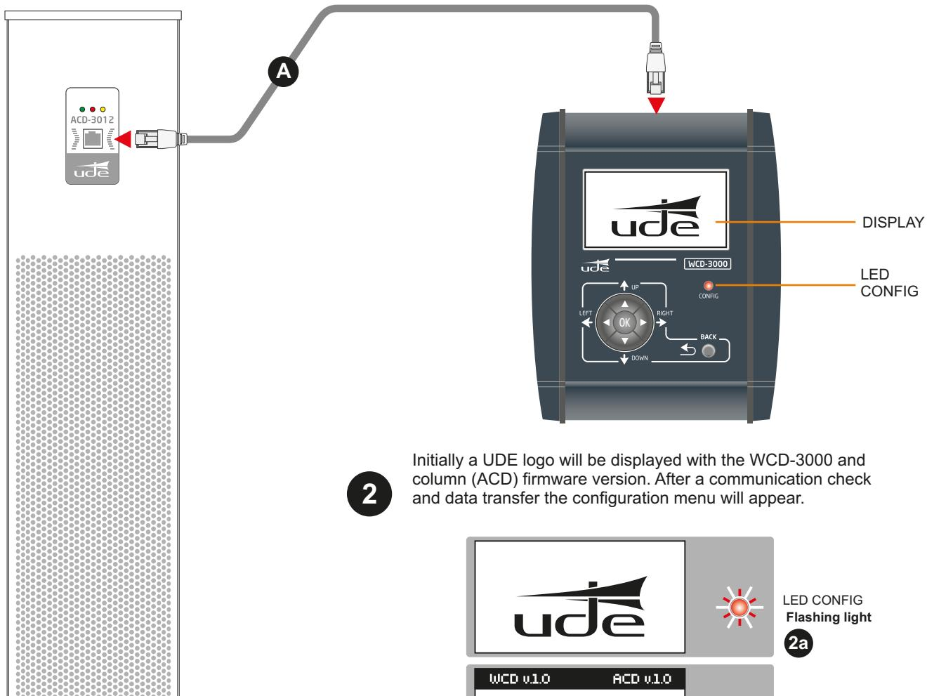
Initially a UDE logo will be displayed with the WCD-3000 and column (ACD) firmware version. After a communication check and data transfer the configuration menu will appear.
