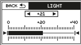
Back light menu control allows setting manually the backlight brightness of the LCD screen.
