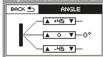
The aiming angle menu allow to set electronically the inclination angle of the beam. The configuration total range is from -45 to +45
