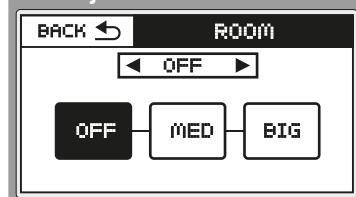
By using the ROOM option, the feedback suppressor can be activated depending on the size of the room where the sound reinforcement is being installed:
