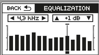
In the equalization menu, it allow to manage 15 frequency:
